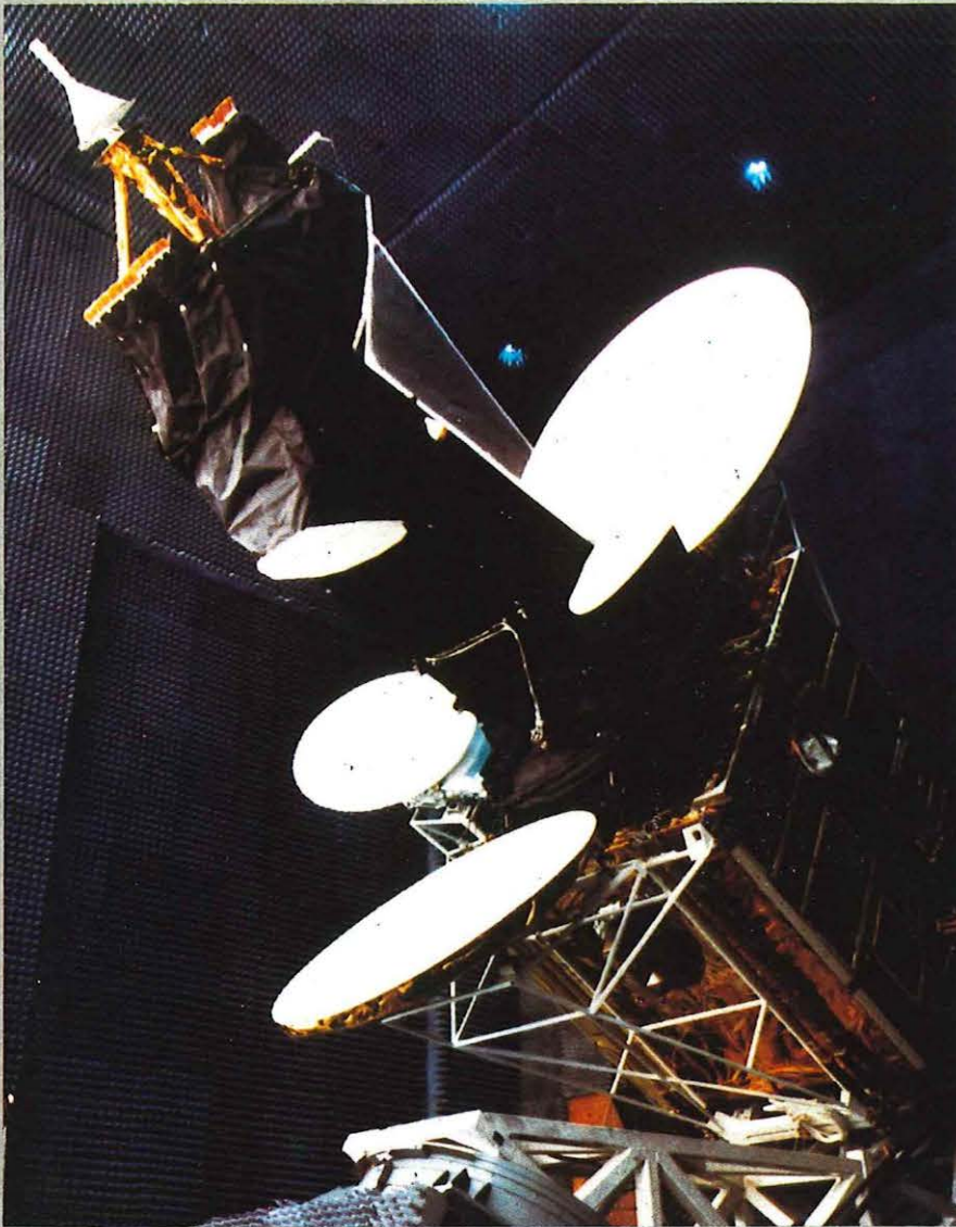
The Intelsat V spacecraft – minus solar panels – undergoes antenna pattern measurements. Due for launch within the next six months, the satellite has a capacity of about 12,000 circuits and two television channels.
