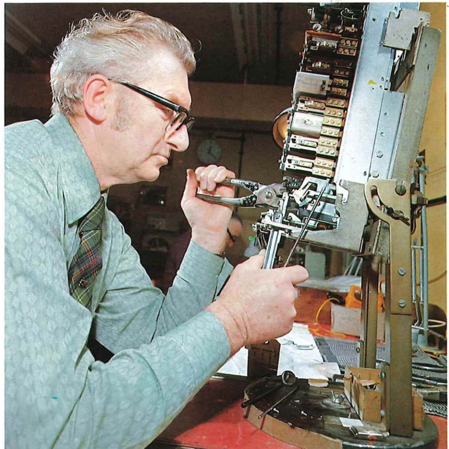
At City Telephone Area's piece part depot, a senior technician replaces a bearing pin in a 2000-type selector.
