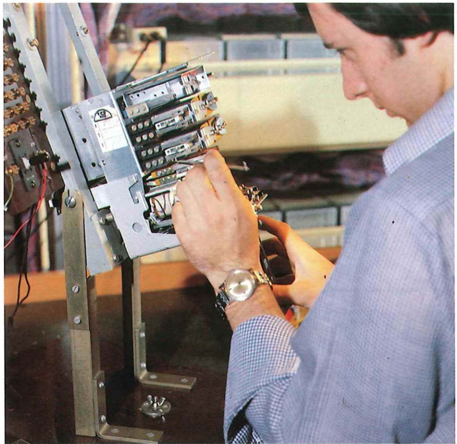
Trainee technician Alastair Carruthers adjusts a relay spring on a 2000-type two-motion selector at an exchange test bench.
