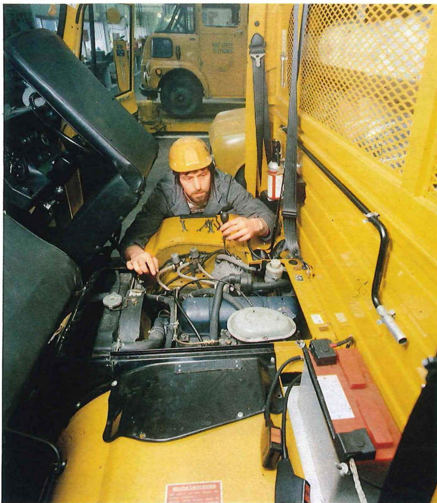
Telecommunications vehicles fuelled by liquid petroleum gas are on trial in the Leeds area. Here senior technician John Scott makes an adjustment to the gas regulator in one of them.
