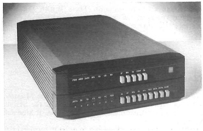
The 4142 TCX modem can be configured as shown with the 4062X six-channel synchronous time-division multiplexer, or as a stand-alone unit
