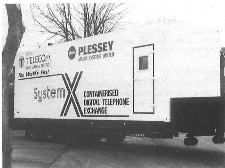
Figure 1—Containerised System X exchange being delivered to Felixstowe Dock site
