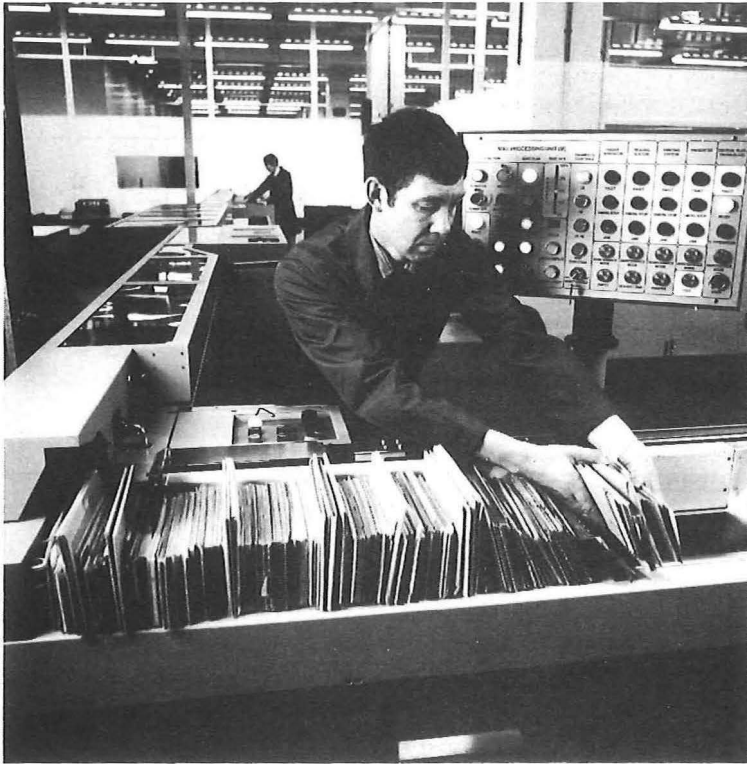
Figure 2—Optical character recognition coder/sorter system
