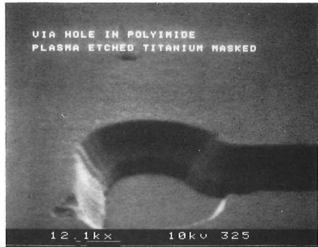
Fig. 5—Scanning electron micrograph of interconnect via
