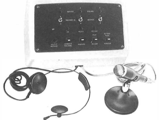
Fig. 7—RISC control panel used at small recording centres
