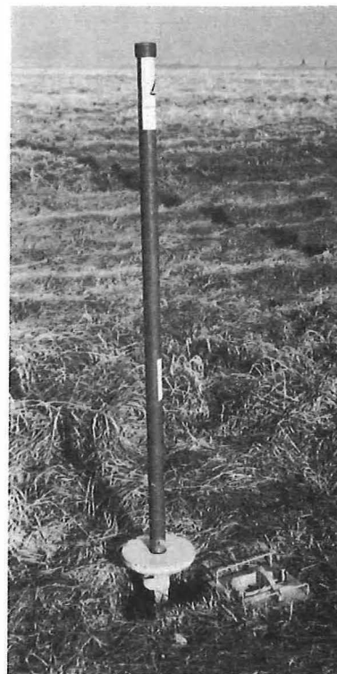
(b) Insulated slide hammer, anchor driven fully home
