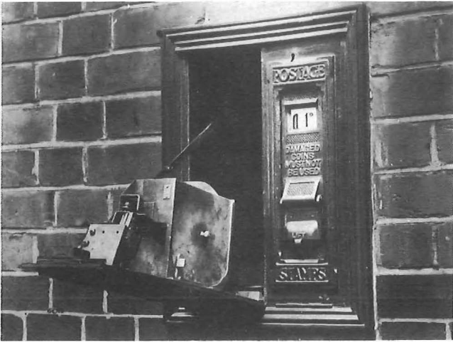
Two Type B machines wall mounted in cast-iron case (Type F)
