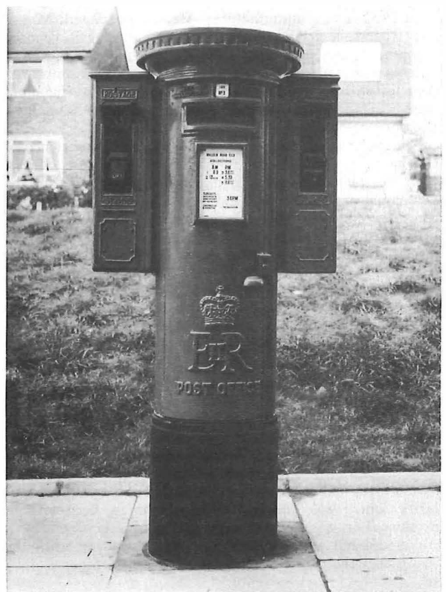
Pedestal-mounted cast-iron case ( Type K ) housing ½d and 1d Type B machines. Door to cash boxes is separate from machines
