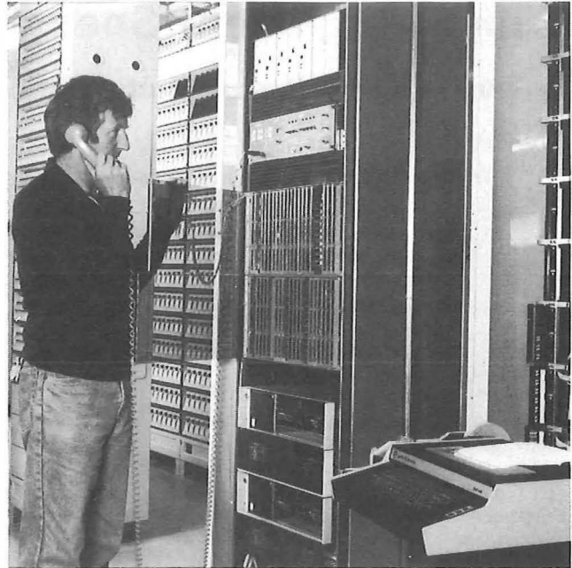
FIG. 4—Celtic 2G terminal with associated teleprinter need at the moment, BTI have evaluated it as satisfactory for use in the PSTN.
