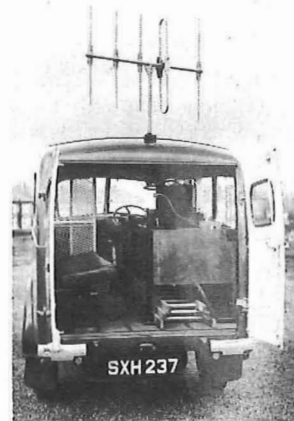
Interior of new radio investigation vehicle showing operating position, apparatus cabinet and aerial support
