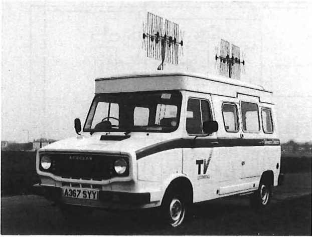
FIG. 2—Detection vehicle showing aerial arrays
