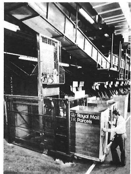
FIG. 33—An experimental automatic container filler on trial at Cardiff PCO
