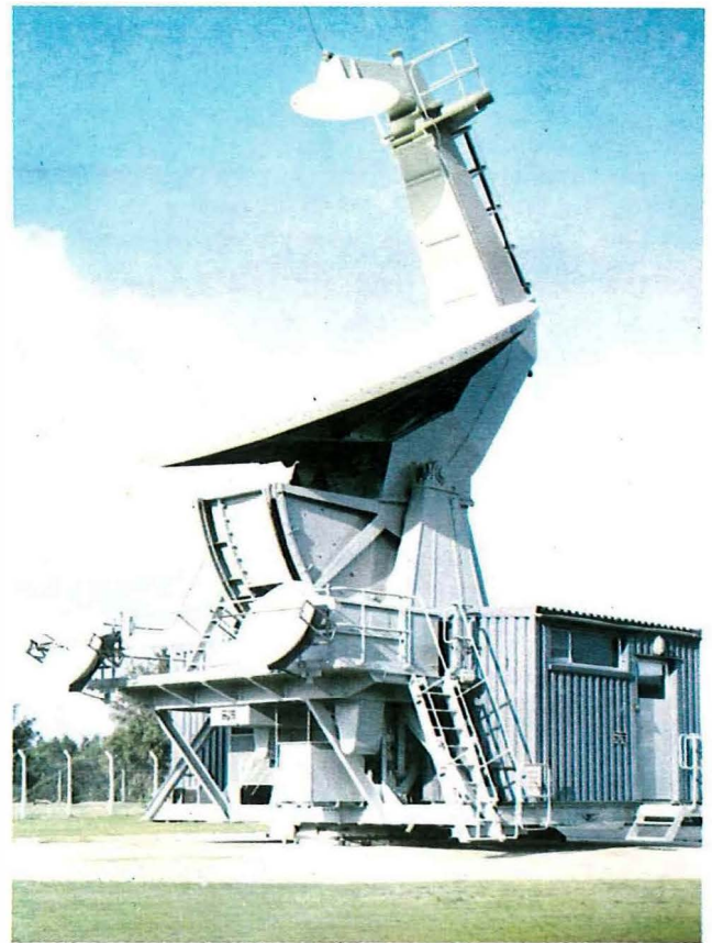
The Martlesham 6 m diameter steerable aerial used for propagation studies
