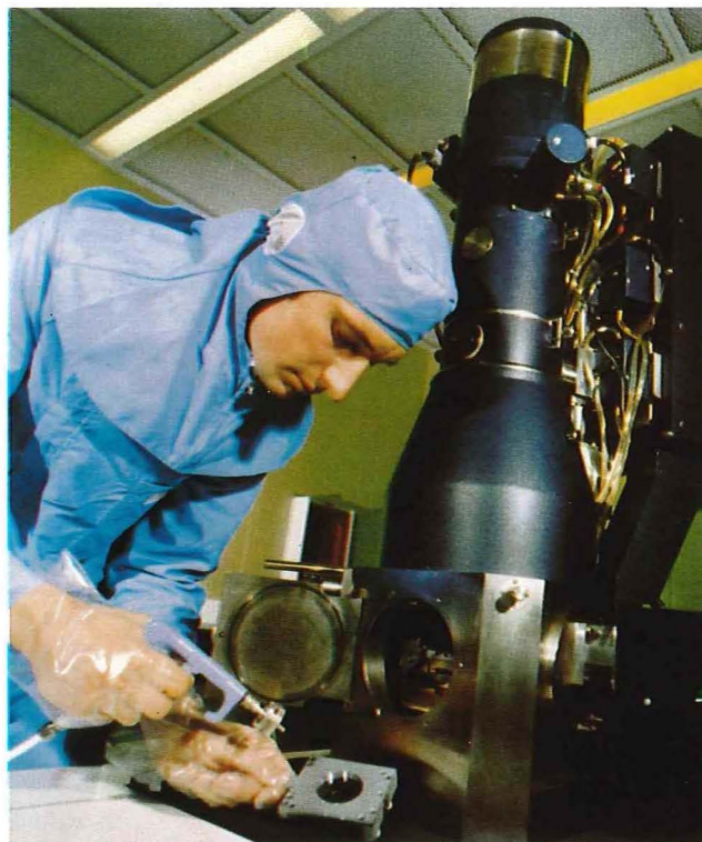
Loading an electron beam micro-fabricator used in the manufacture of integrated circuits
