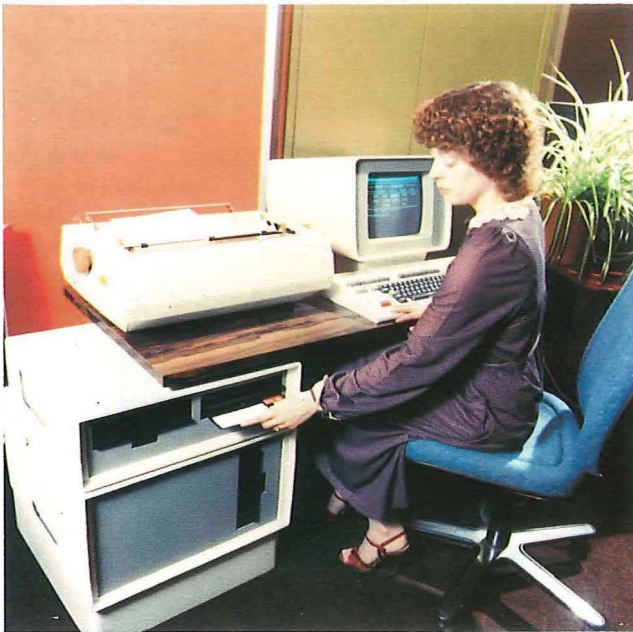
A demonstration Teletex terminal operating the full 308-character alphabet for 40 latin-based languages
