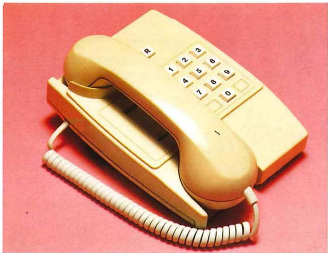
Note: Modern electronic press-button telephones (with loop-disconnect (LD) or multi-frequency (MF) signalling) can be used with key systems as well as the multi-key terminals
