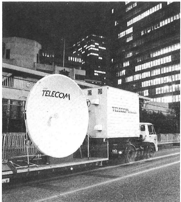
Road-transportable small-dish earth station
