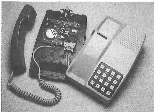
FIG. 3—Microtel I/TMS, BTRL's first telephone containing a CMOS microprocessor
