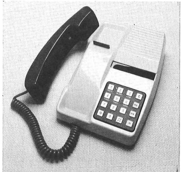
FIG. 2—Microtel I, BTRL's first microprocessor-controlled telephone
