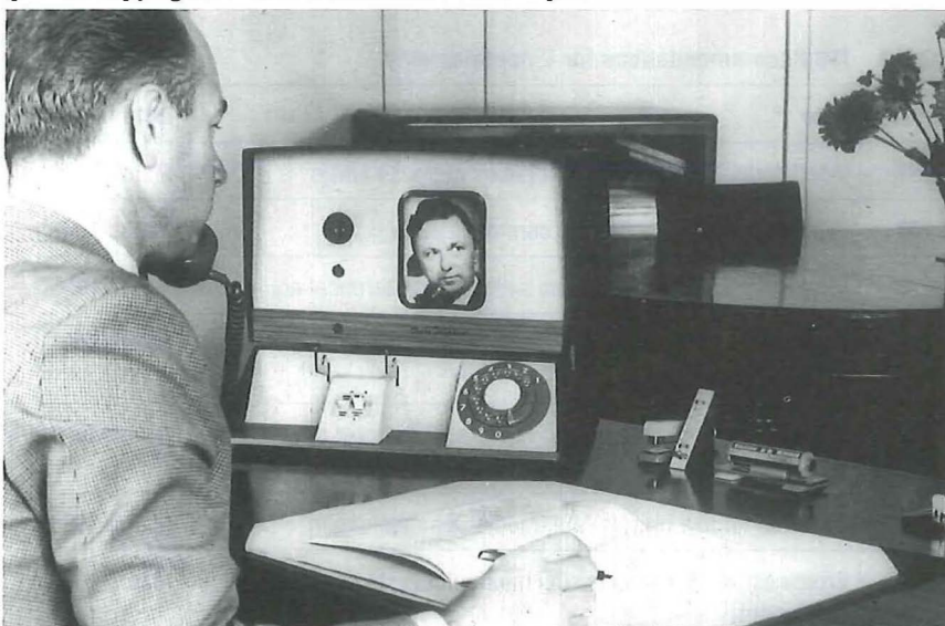
Figure 1—An early videophone prototype, using a close-up view of the face (picture copyright British Telecommunications plc)
