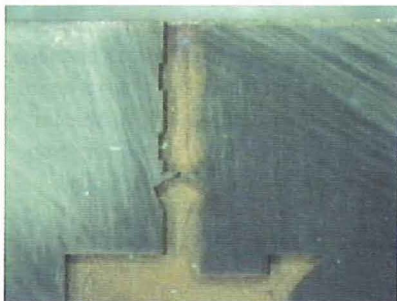
(a) Fibre and ball lens alignment
