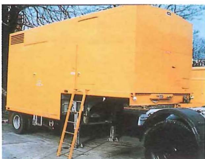
Figure 6—500 kW mobile gas turbine
