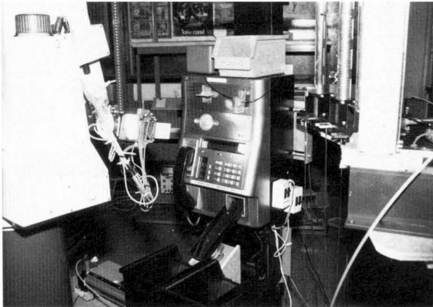
Figure 4—Rodless cylinder 'shuttles' collection boxes to refund chute for mis-validated and returned coins
