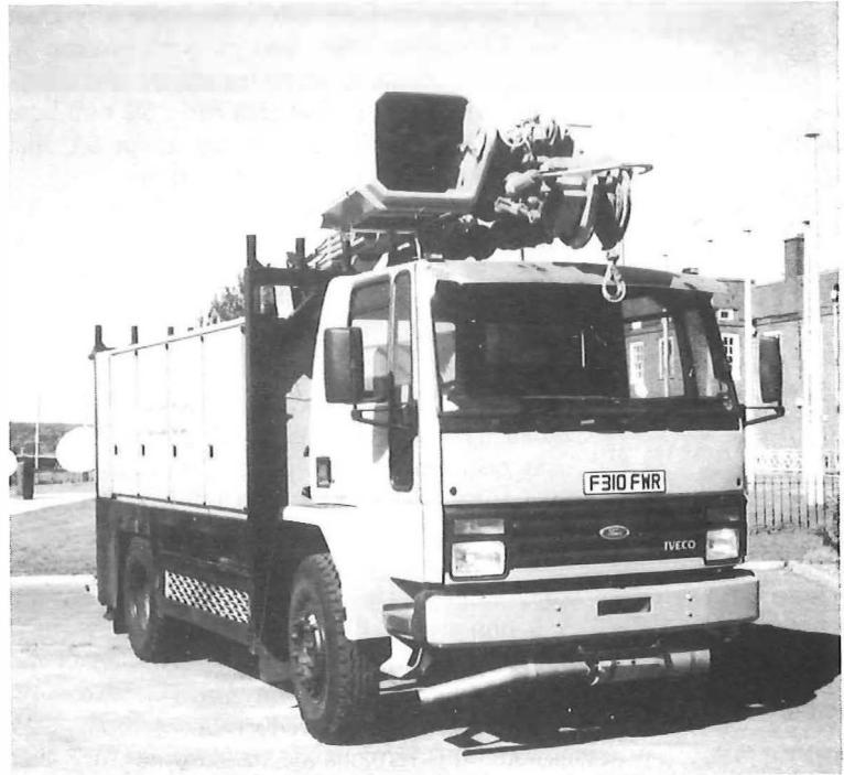
Figure 10 Modern pole erection unit
