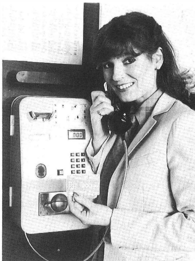
Cardphone—public telephone which takes plastic cards instead of coins.
