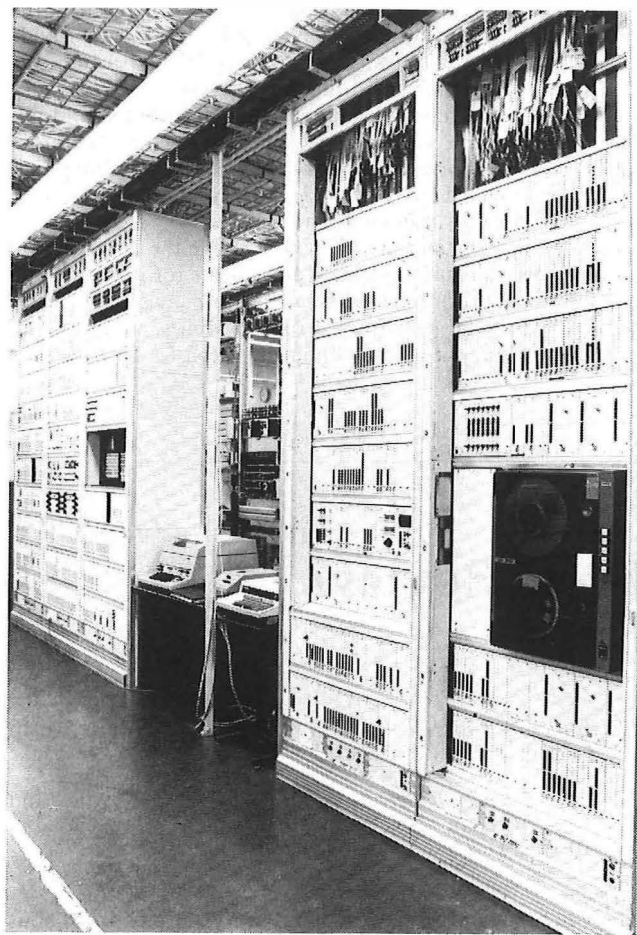
FIG. 1—TXE4A test bed (Model B) equipment. This equipment at Armour House, London, is used to provide test-bed facilities for future developments
