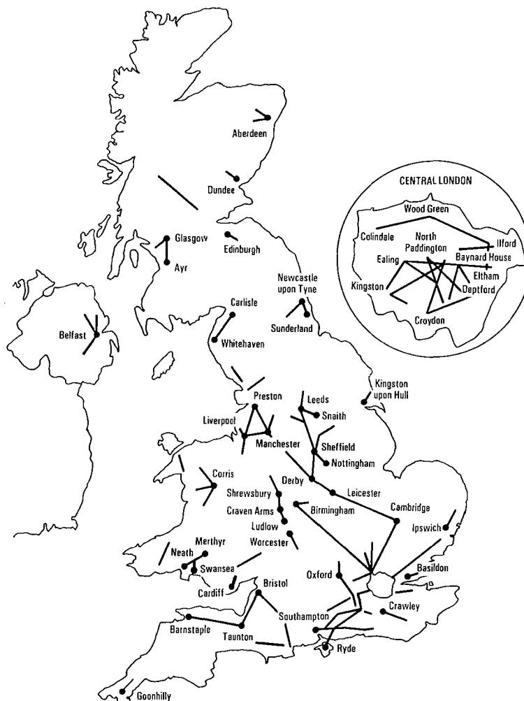
British Telecom's Lightlines network—4000 fibre kilometres already installed, and a further 22 000 fibre kilometres currently on order.
