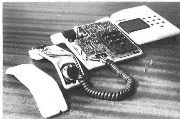
FIG. 3—Interior of case and handset
