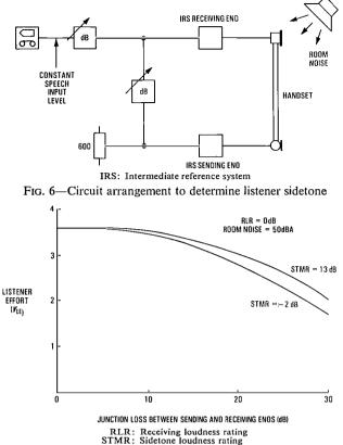
FIG. 7-Effect of sidetone level on listener opinion score
