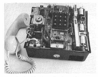
FIG. 10-Coin Telephone No. 23 mechanism
