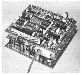
FIG. 5—Complete viewdata and teletext module Photograph by courtesy of Mullard Ltd.
