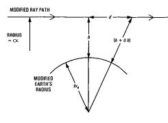
(b) Modified straight-line-path profile FIG. 10—Radio wave path profile
