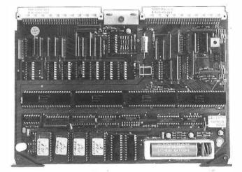
FIG. 7—Coin Telephone No. 22B processor board showing lithium battery
