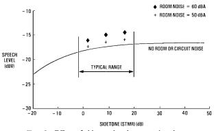
FIG. 5-Effect of sidetone level on speech voltage
