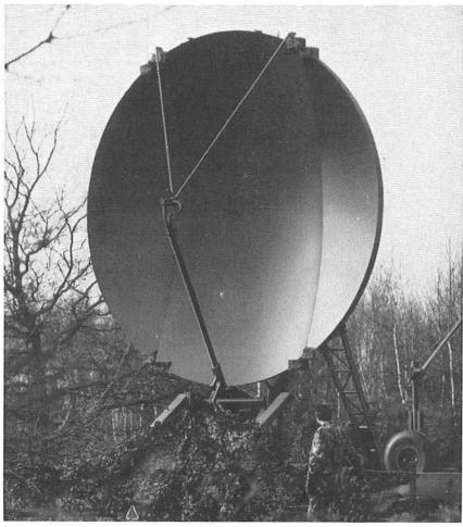
Equipment mobility is vital to an army in the field. This ccmpact, self-contained tropospheric scatter system has a folding reflector allowing extremely rapid deploy and tear-down times. The entire system is fully transportable by road or air.
