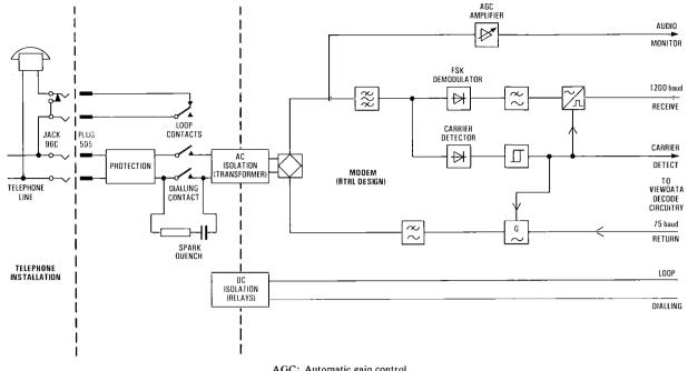
AGC: Automatic gain control FSK: Frequency-shift keying FIG. 3—Block diagram of line interface circuitry
