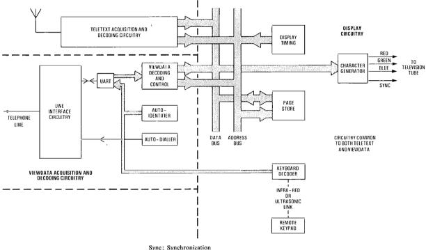
Sync: Synchronization UART: Universal asynchronous receiver transmitter FIG. 4—Block diagram of complete viewdata terminal
