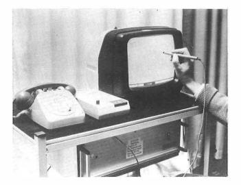
FIG. 1—CYCLOPS audiographic terminal used in the Open University trial, 1981-82
