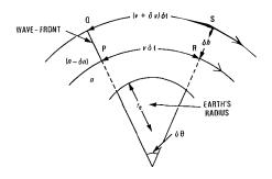
FIG. 11-Effect of refractive index on radio wave path
