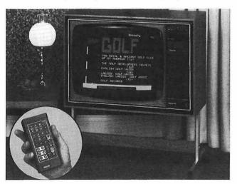
FIG. 1-Domestic terminal equipped for Prestel, teletext and normal television reception Photograph by courtesy of Philips Ltd.
