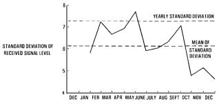
Note: Path details of this system are given in Table 2 FIG. 7—Monthly standard deviation of received signal level
