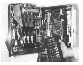
FIG. 5-Tester 297 in use with Coin Telephone No. 22B
