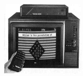
FIG. 7-Prestel adapter with normal domestic television Photograph by courtesy of Zycor Ltd.
