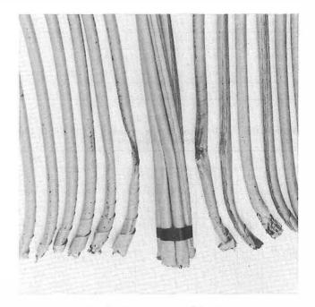
FIG. 2-Damage to coaxial pairs
