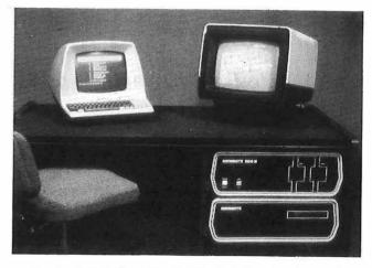
FIG. 8-Information provider intelligent inputting terminal Photograph by courtesy of Metrotech Ltd.
