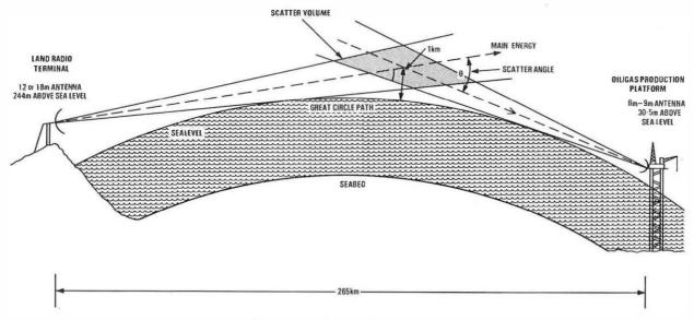
FIG. 3—Path geometry of tropospheric-scatter propagation
