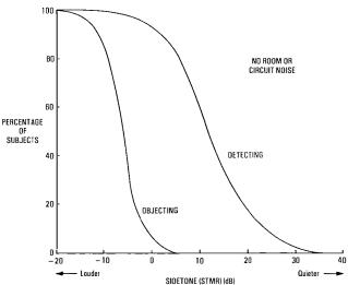
FIG. 4—Effect of sidetone level on detectability and objectionableness
