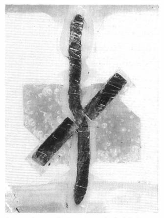
FIG. 2—Section through IDT termination showing deflection of tag and indentation in wire
