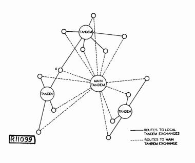
Fig. 11 has been developed by the addition of several small tandem exchanges, so located that they relieve the main tandem exchange of much of the semi-local traffic passing between the exchanges which they serve. This arrangement permits the main tandem exchange to deal primarily with calls passing across the main area and effects a further saving in junction cabling.
