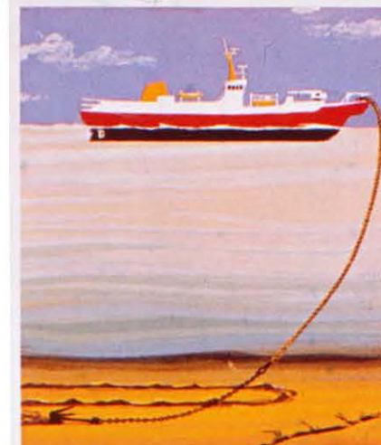
The cableship is fishing for a faulty cable with a grapnel.
