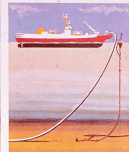
The fault has been cut out and a new cable joined. The ship is now paying out cable on its way back to the buoy. The buoy is about to be picked up and the other cable end recovered.
