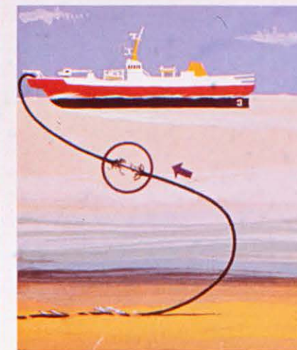
The faulty end has been retained and the cableship will pick up the cable until the fault is on deck.
