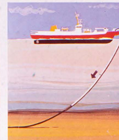
The fault has been cut out and a new cable joined. The ship is now paying out cable on its way back to the buoy. The buoy is about to be picked up and the other cable end recovered.
