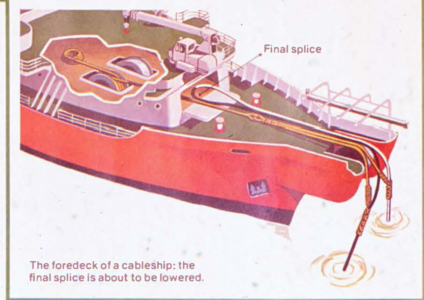
The fault has been cut out and a new cable joined. The ship is now paying out cable on its way back to the buoy. The buoy is about to be picked up and the other cable end recovered.
