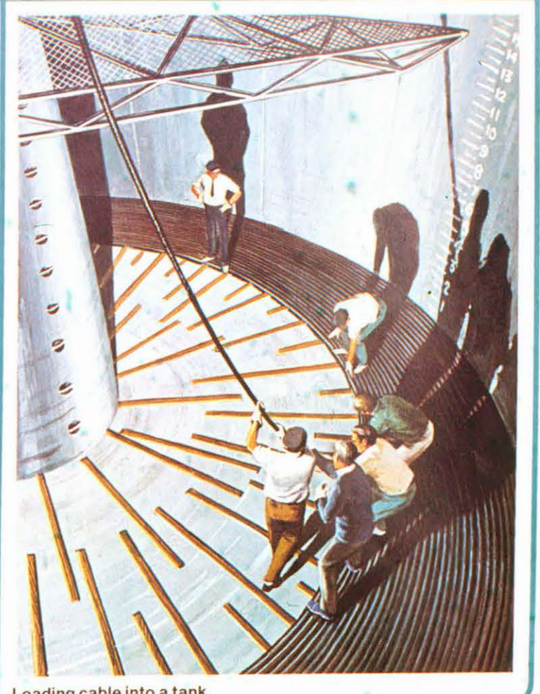
Loading cable into a tank.
