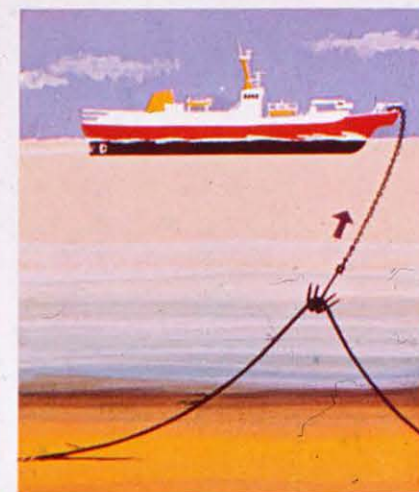
The faulty cable has been found and is being raised.
