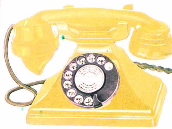
Plastic telephone with improved transmitter that solved the handset problem, 1929.
