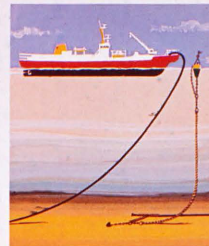
The cable has been cut and tested and the good end has been dropped and buoyed.
