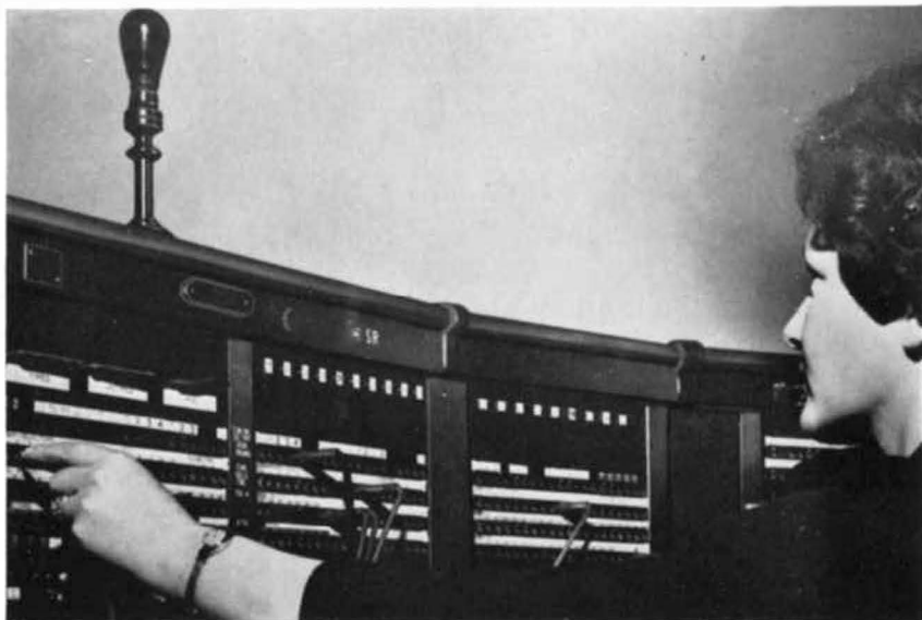
999 position at an exchange switchboard showing lamp
