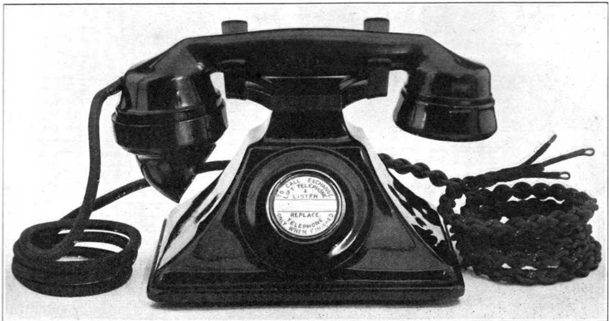
FIG. 1.—THE NEW C.B. MICROTELEPHONE.
