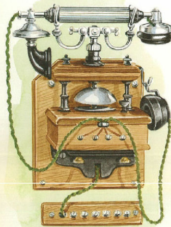
Handsets gave some freedom of movement to telephone users, but early handsets proved unsuccessful as the exchange system grew.
