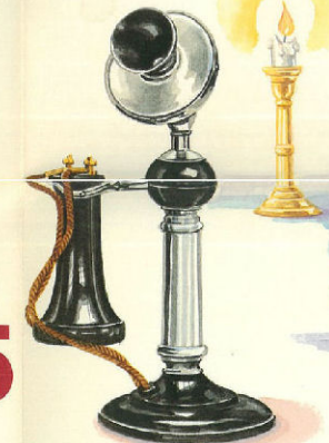
Called 'candlestick' telephones because of their shape, these were used from the 1900s for over half a century. Later models had dials.
