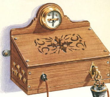
Callers spoke into the fretwork front of this telephone.
