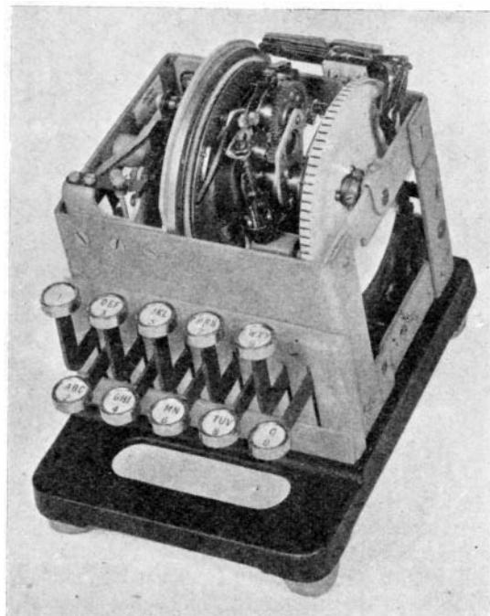
FIG. 335. KEYSENDER WITH COVER REMOVED
