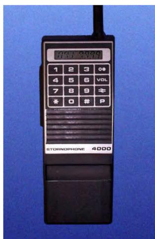
The operation of the Stornophone 4000 hand portable radio (left) is explained. This was later superseded by the Brunel hand portable radio (right) with a further increase in power, but a less efficient antenna. Despite the warning in the film on the radio's fragility the Brunel is in fact a robust piece of equipment and is considerably more powerful than its modern cellphone counterparts.
