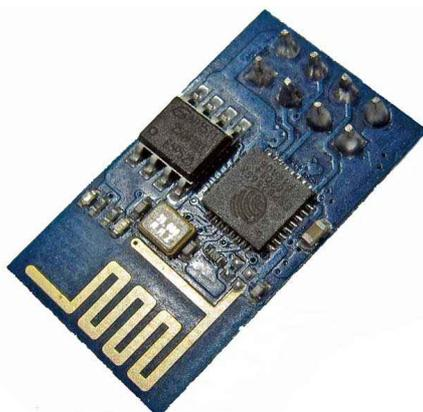
This “ESP-01” is the first and most popular version of the board. It has a printed antenna and an 8-pin header block to allow it to easily be plugged-in to the main board. The module is readily and cheaply available from many China Ebay vendors and various websites.
